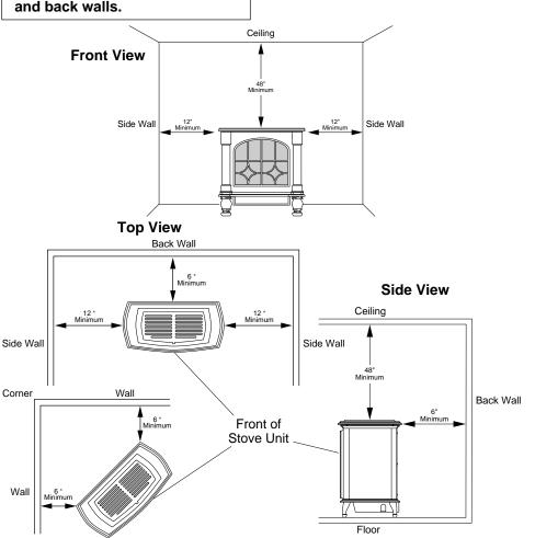
Figure 4 - Minimum Clearance to Walls and Ceiling (Stove May Vary Depending on Model) Continued
